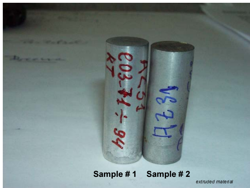
Figure 4: Outlines of two AZ31 specimens after the compressive tests. (Sample #2 was measured at 150 °C).
