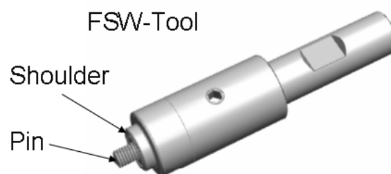
Figure 1. FSW tool pin and shoulder.
