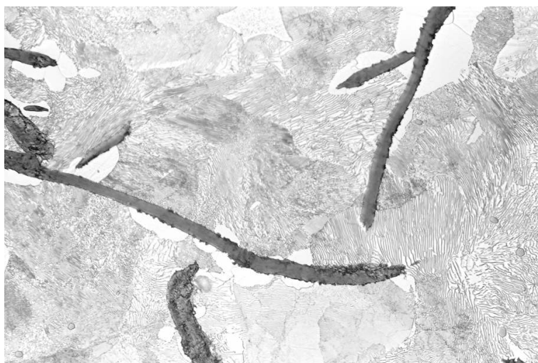
Microstructure GJL, 100% Perlite, 500 x
