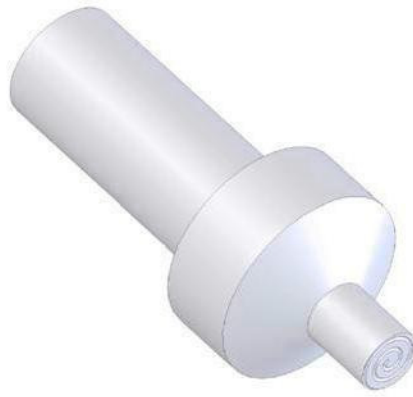
Figure 2: Schematic of HFDB tool with engraved shoulder.
